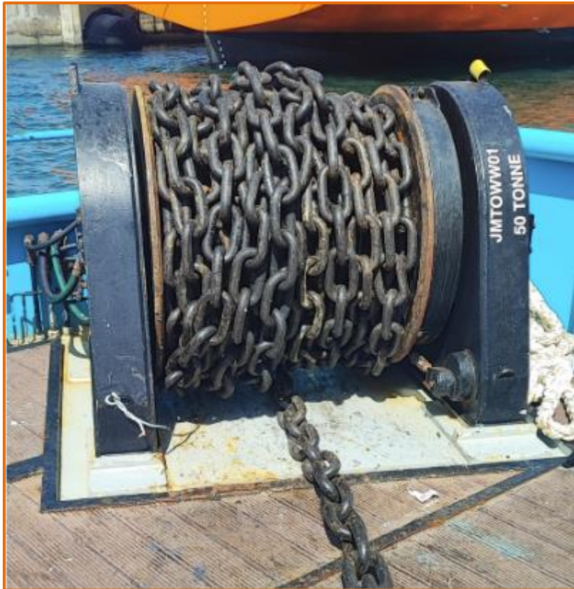
Figure 7: 32mm chain spooled onto the main winch drum.
