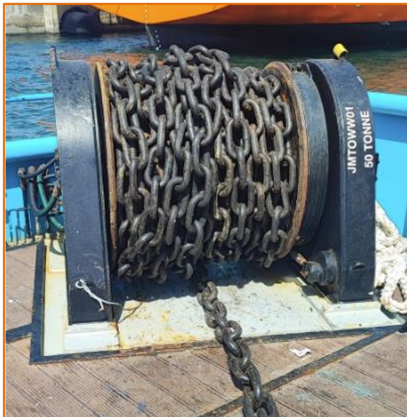
Figure 7: 38mm chain spooled onto the main winch drum.
