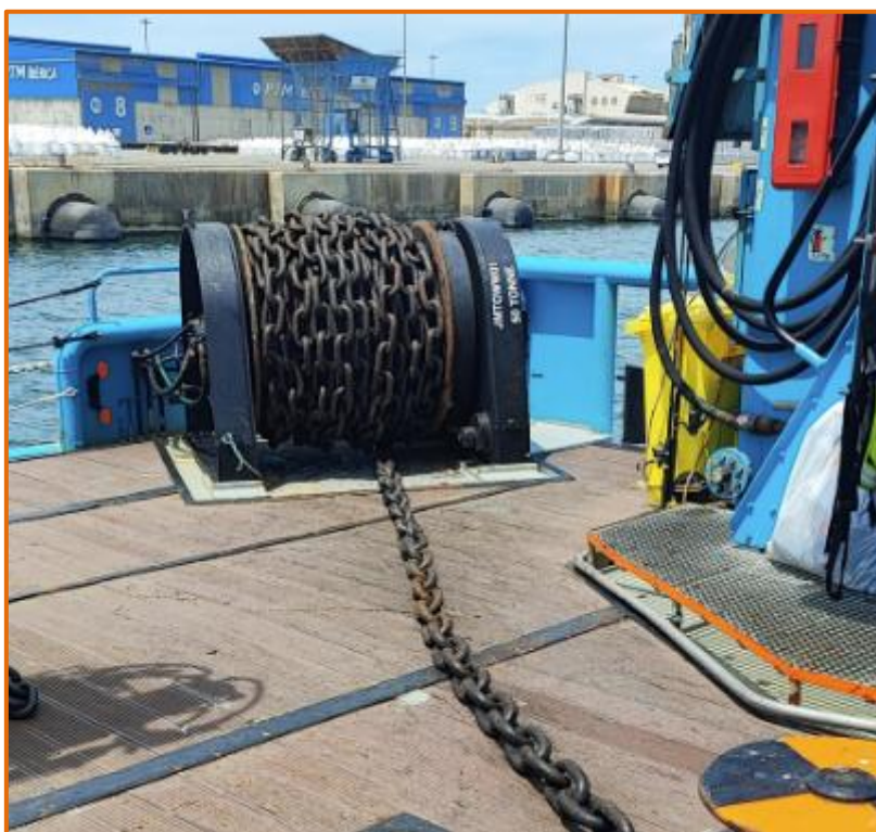
Figure 7: 36mm chain spooled onto the main winch drum.
